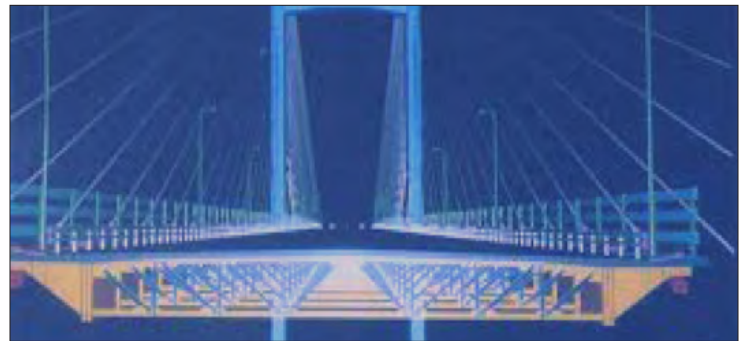
Figure 13 - Steel Box Section for Longer Spans
